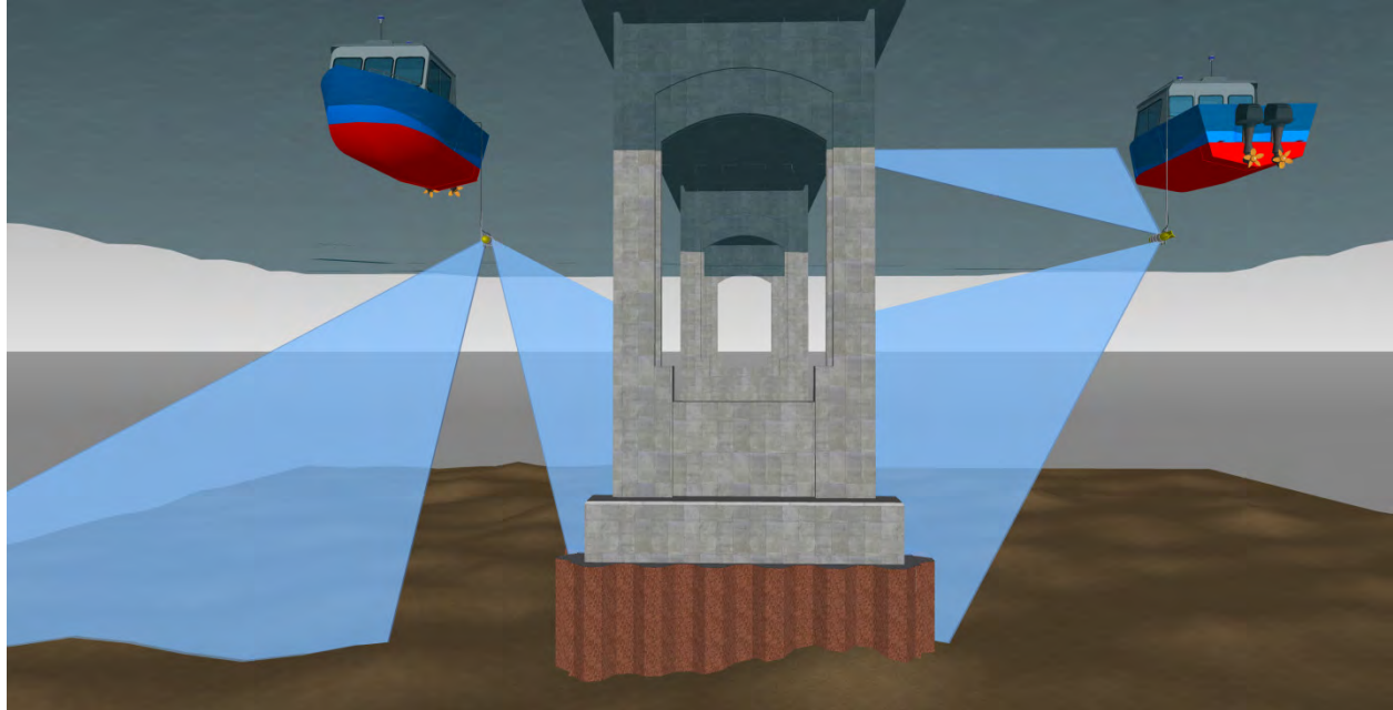
Figure 14. Graphic. Side-scan sonar mounting positions for structural imaging (right) and bottom scanning (left).
