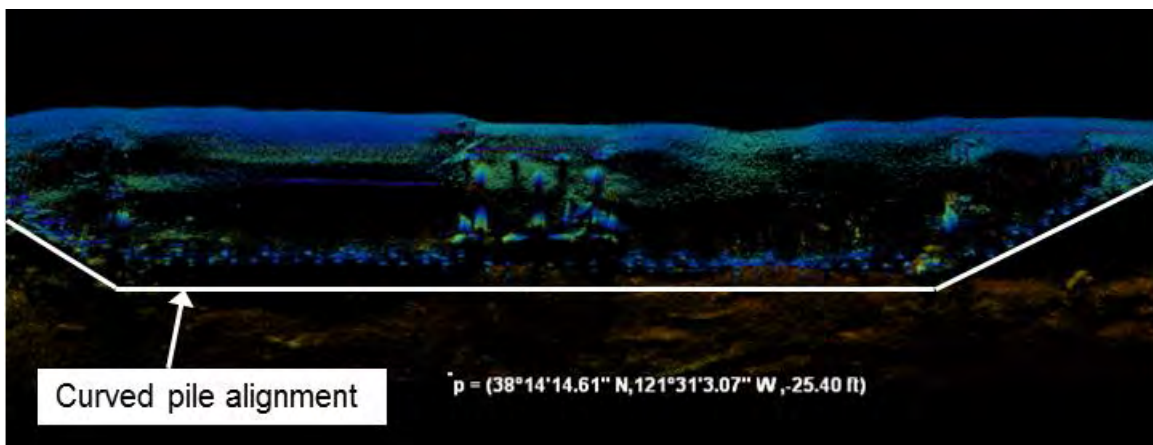
Figure 27. Image. Curved pile alignment in plan view (Georgiana Slough).
